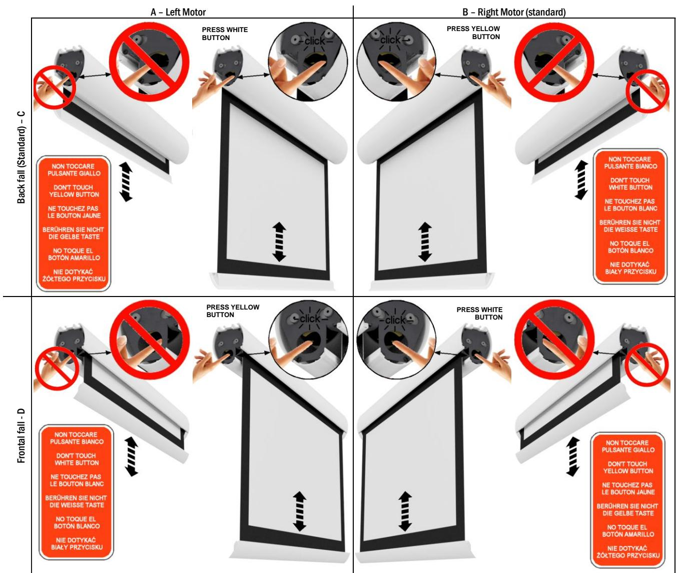
**PROGRAMMING END STOPS MOTOR SOMFY RTS 230V 50Hz/120V 60Hz (procedures already carried out in factory, SHOULD NOT be performed by unauthorised personnel)**
