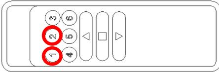
Before start the programming choose the engine you want to program with the number button, 1 – fabric motor, 2 – masking motor.
