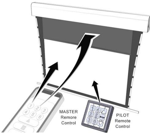
**MASTER** remote: must be used by technical staff; it enables the memorization of upper, lower and intermediate end stops of the two individual maskings
