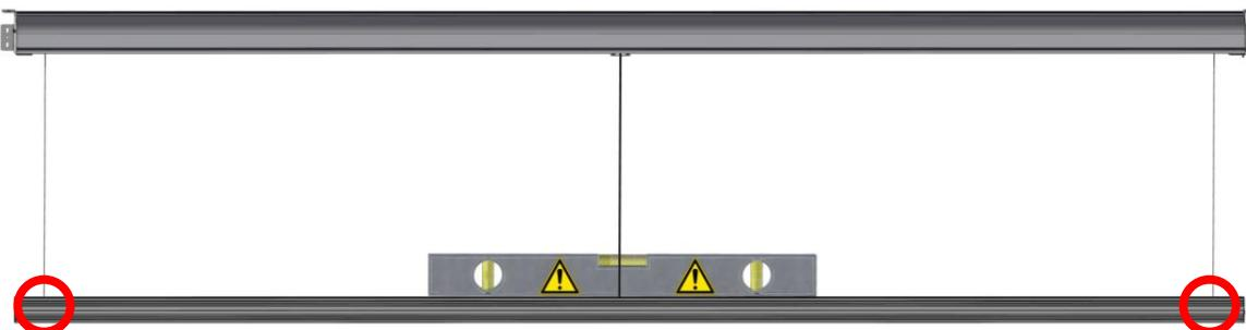
**Fix the screen exclusively under the bar, not on the side in front.**
