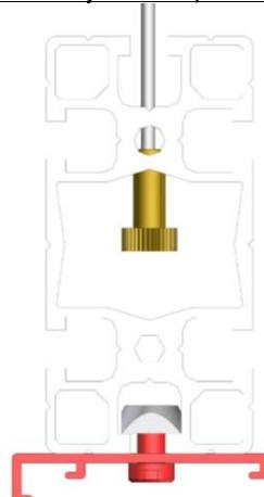
Secure the screen brackets on the nut M6 already inserted in the bar. Subsequently anchor the screen on the brackets.
