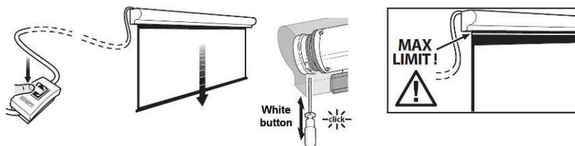
**3**–Move the projection fabric in the up end position and release the yellow button
