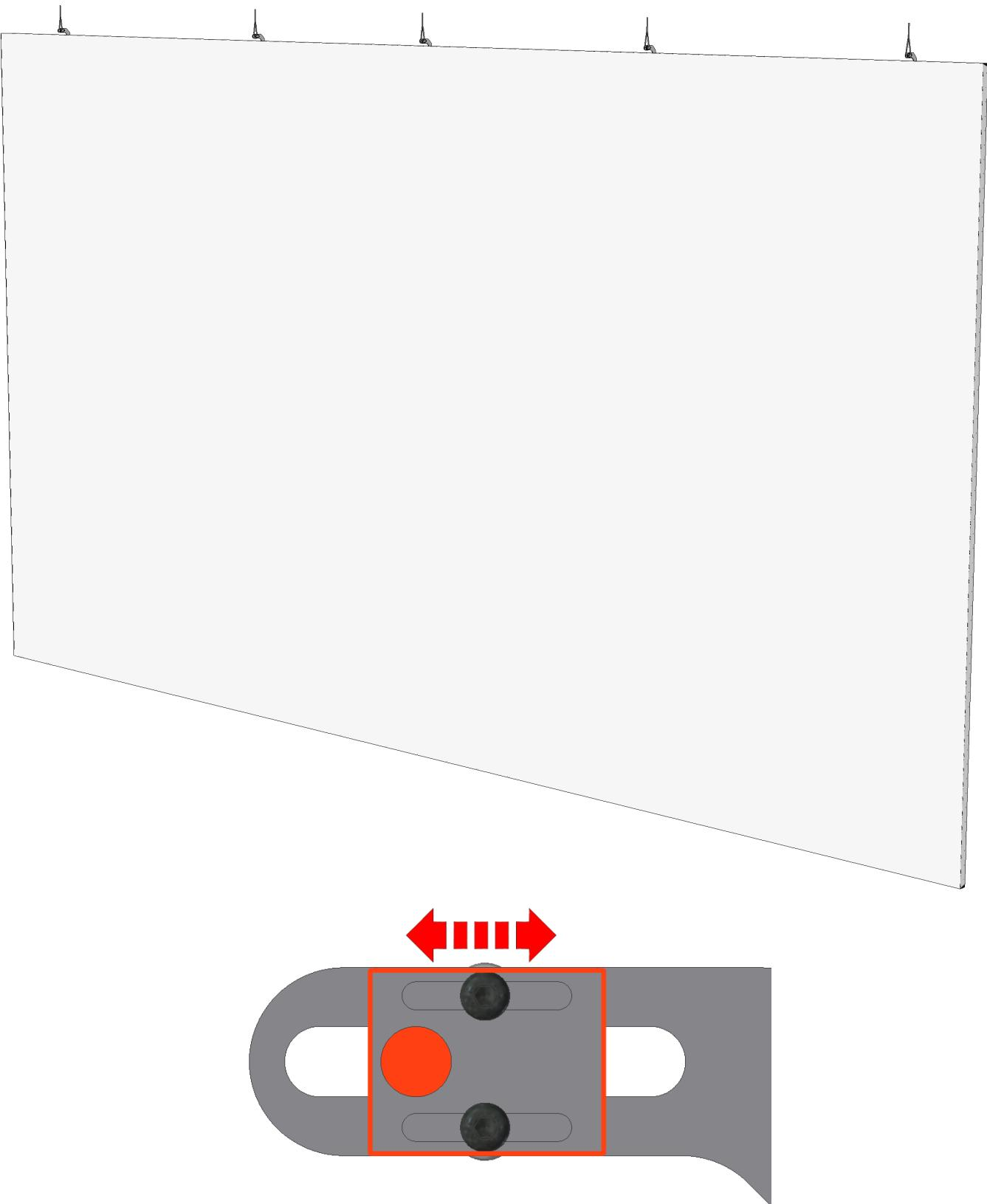
Move the small bracket left and right to adjust the horizontal plane of the screen.
